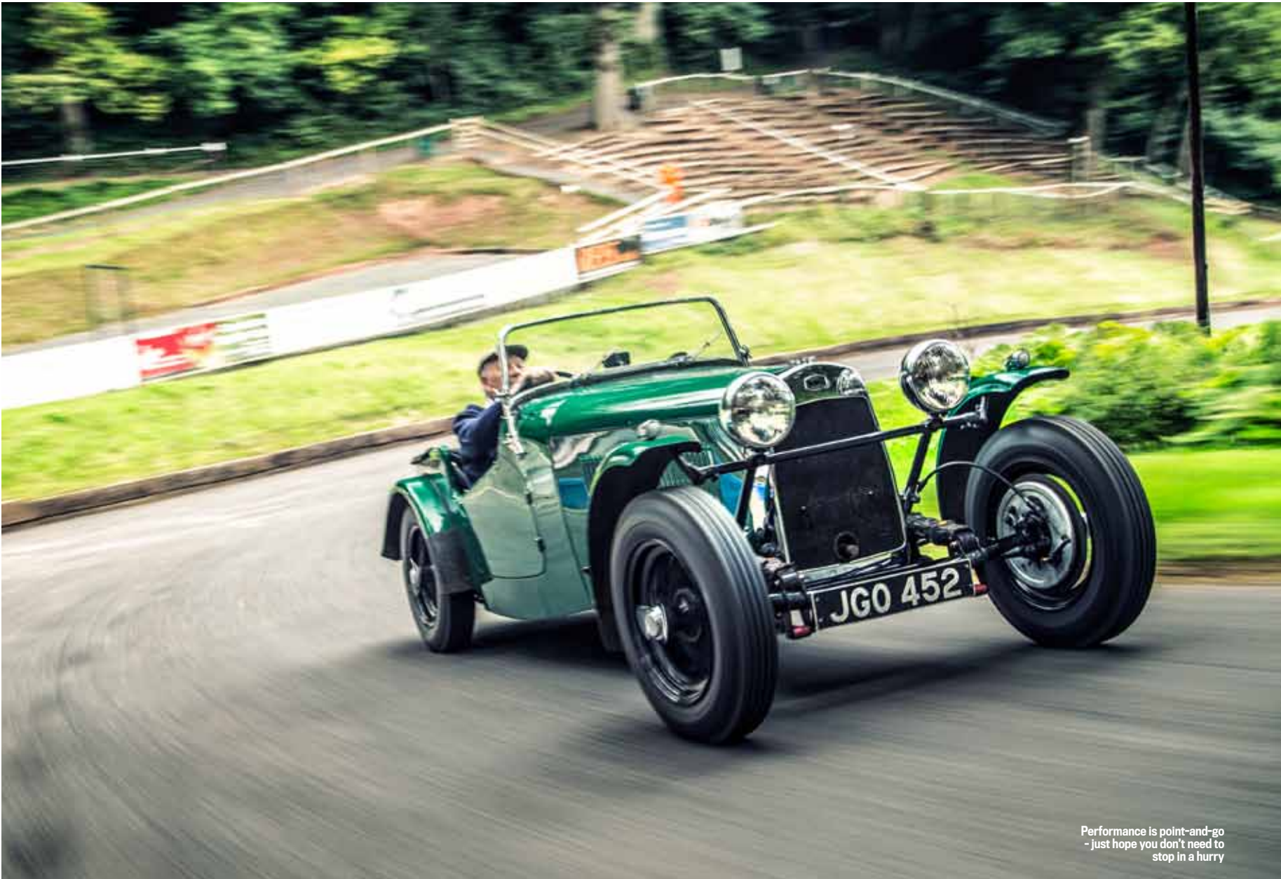
1496cc Singer motor yields a mere 62bhp, but at 737kg the HRG is the lightest car here
